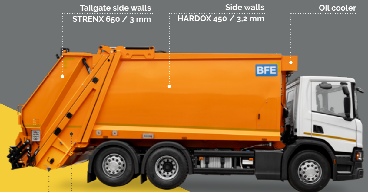
Tailgate bottom side walls STRENX 650 / 6mm
